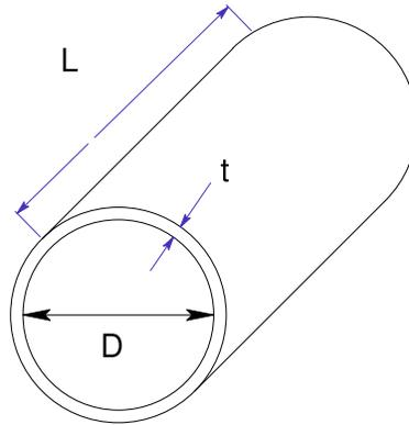
It is assumed that the flow is laminar and the fluid is Newtonian, such that the fluid displays a linear dependence of the shear stress on the shear rate. The experiment is conducted with fluid in between two concentric cylinders with one cylinder fixed. Since the radius,  $D/2$ , is much larger than the gap width,  $t \ll D/2$ , the flow is essentially Couette flow. In the assignment, the parameters are as given in table 1.
