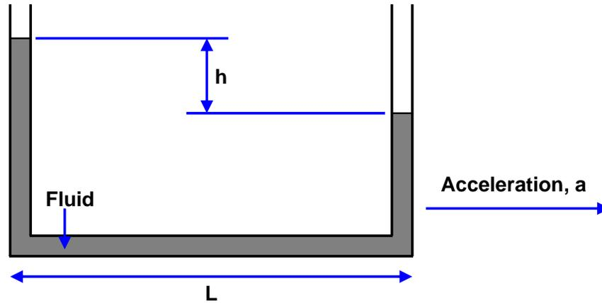
When the vehicle is accelerating at a constant rate,  $a$  (in  $m/s^2$ ), the difference in the elevation of the levels in the manometer is  $h$ . What is the relation between  $a$ ,  $h$ ,  $L$  and the acceleration due to gravity,  $g$  ?
