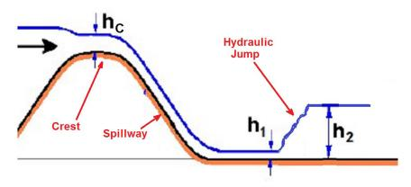
Since the flow over the crest is choked, it follows that the velocity,  $u_c$ , of the flow at the crest is given by  $(gh_c)^{1/2}$  and therefore the volume flow rate per unit breadth, Q, is
