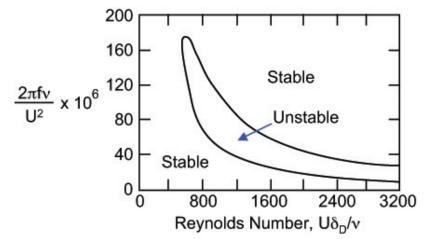
Using the solid, theoretical curve find the distance from the leading edge of the plate to the point where transition to turbulence begins for a flow of water ( $\nu = 10^{-6} m^2/s$ ) when U = 2 m/s. What is the frequency of the most unstable disturbances (in Hz) under these conditions?
