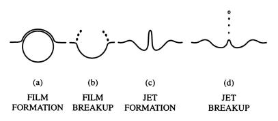
Figure 1: Stages of a bubble breaking through a free surface.
