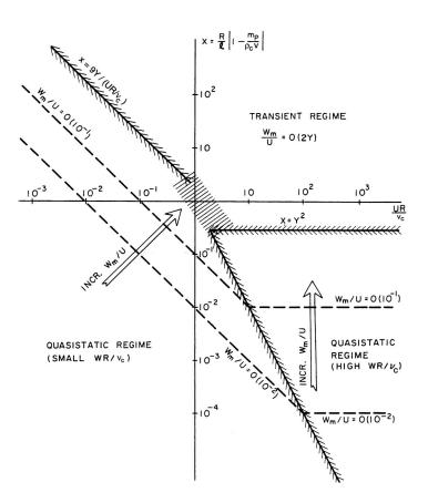
Figure 1: Schematic of the various regimes of relative motion between a particle and the surrounding flow.
