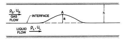
Figure 1: Sketch showing the notation for stratified flow instability.
