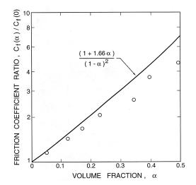
Figure 1: The ratio of the base curve friction coefficient at finite loading,  $C_f(\alpha)$ , to the friction coefficient for the continuous phase alone,  $C_f(0)$ . Equation ?? (line) is compared with the data of Lazarus and Neilsen (1978).
