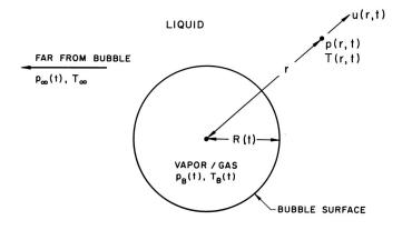
Figure 1: Schematic of a spherical bubble in an infinite liquid.
