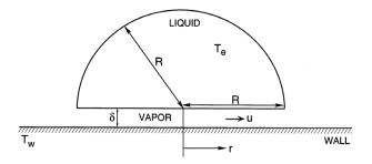
Figure 1: Hemispherical model of liquid drop for the Leidenfrost analysis.
