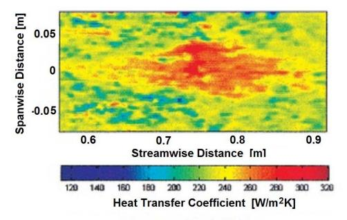
Figure 1: Liquid crystal visualization of the heat transfer and therefore the shear stress under a turbulent spot. Photograph by Guo *et al.* (2000).
