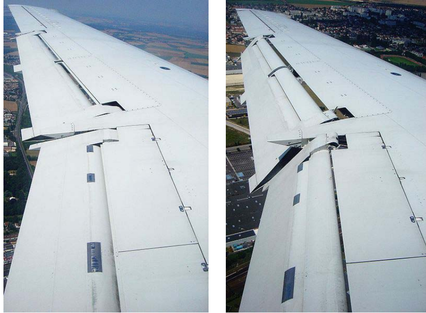
Figure 4: Wing of an Embraer ERJ 145 showing the flaps slightly extended (left) and fully extended (right).
