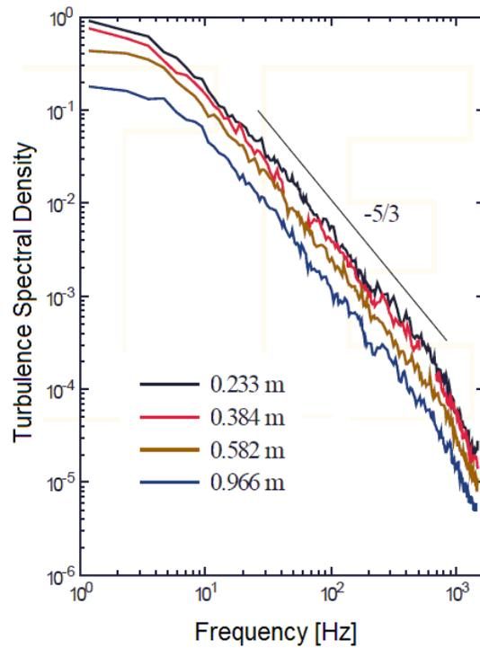
Figure 2: Turbulence spectra measured in a wind tunnel by Witter *et al.* (2013). Four spectra of the longitudinal velocity are shown for four different heights above the floor of the wind tunnel as shown.
