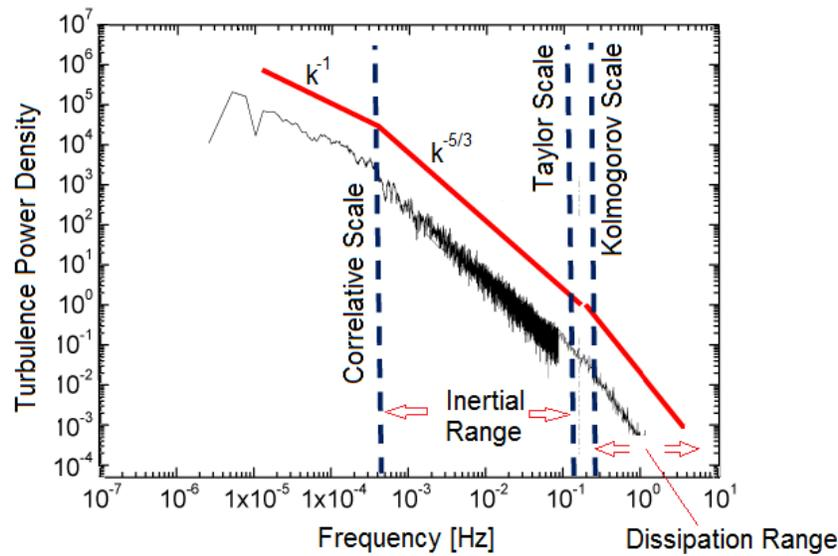
Figure 1: Characteristics of a turbulence spectrum. Adapted from Bruno and Carbone (2013).
