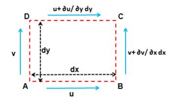
Figure 2: Circulation around an infinitesmal element.
