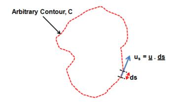
Figure 1: Circulation around an arbitrary closed contour in a flow.
