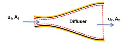
Figure 1: A diffuser with steady, incompressible flow.
