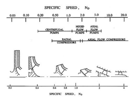
Figure 2: Pump shapes as a function of the specific speed, N (from Sabersky, Acosta and Hauptmann 1989).
