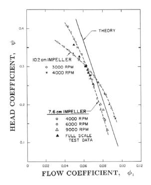
Figure 3: Non-cavitating performance of Impeller IV (7.58 *cm*, with stator) and Impeller VI (10.2 *cm*, without stator) at various rotational speeds. Also shown are full scale test data from Rocketdyne and a theoretical performance prediction (solid line) (from Ng and Brennen 1978).
