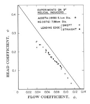
Figure 1: Non-cavitating performance of  $9^{\circ}$  helical inducers of two different sizes and with and without swept leading edges (the 7.58 *cm* inducers are Impellers III and V). Also shown is the theoretical performance prediction in the absence of losses (from Ng and Brennen 1978).
