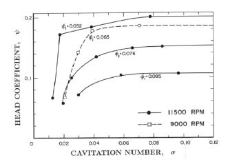
Figure 2: Cavitation performance for Impeller V at various flow coefficients and rotating speeds (from Ng and Brennen 1978).
