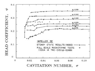
Figure 4: Cavitation performance of Impeller IV at 9000 *rpm* and various flow coefficients. Also shown are full scale test data from Rocketdyne (from Ng and Brennen 1978).
