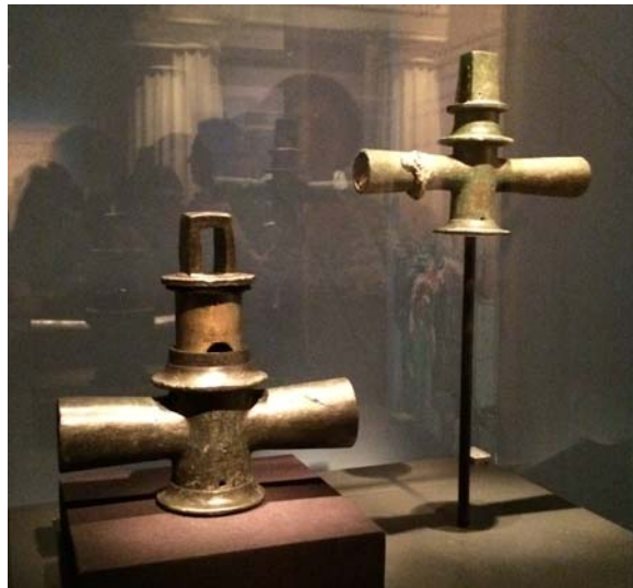
Figure 4: Roman ball valves for water supply systems (from the ruins of Pompeii).
